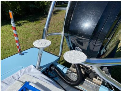
6. Place the poling platform step on your poling platform mounting pads, then insert and tighten the screws, squeezing out excess adhesive sealant until the step is snug to the mounting pads.
