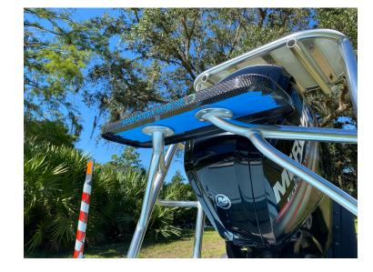
2. Set the poling platform step on your mounting pads and mark the hole locations on the tape with a pencil or sharpie.
